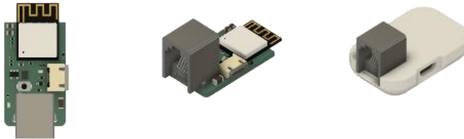
Figure 20. Open-source P1-dongle used. All technical information is available on GitHub
